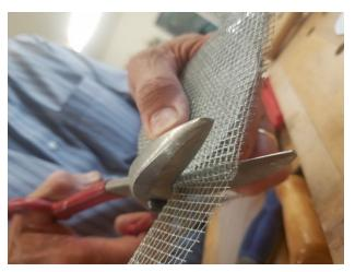
Loren uses a 10" tin snips to cut through 6 layers of #8 hardware cloth. Place a 3 ½" diameter paper template (83mm) on the long strip of hardware cloth approximately 1/4 inch from the end of the cloth. Fold the hardware cloth over the paper template so the fold is at least another ½ inch longer than the paper. (The extra distance between the paper template and the folded edge of the hardware cloth makes it much easier to make an accurate cut.)
