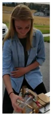
Dylan cuts the bottom from each screened cup using an 18 gauge nichrome wire jig. (Cut the cups outside and don't breathe the nasty fumes of the burning plastic.) We attached the clamps from a manual battery charger **on the 6 volt setting** to the two bolts which hold the nichrome wire.
